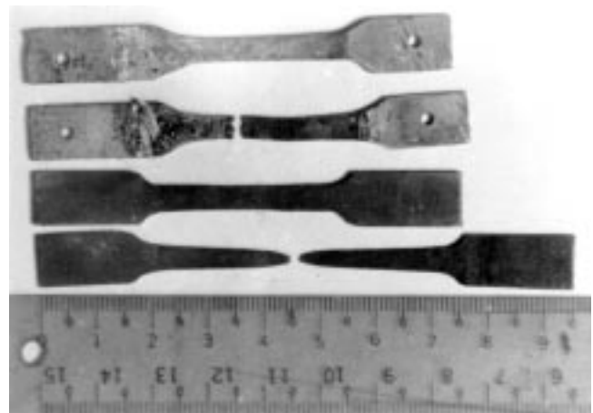
Fig. 3 Specimens before and after tensile test at room temperature in air
